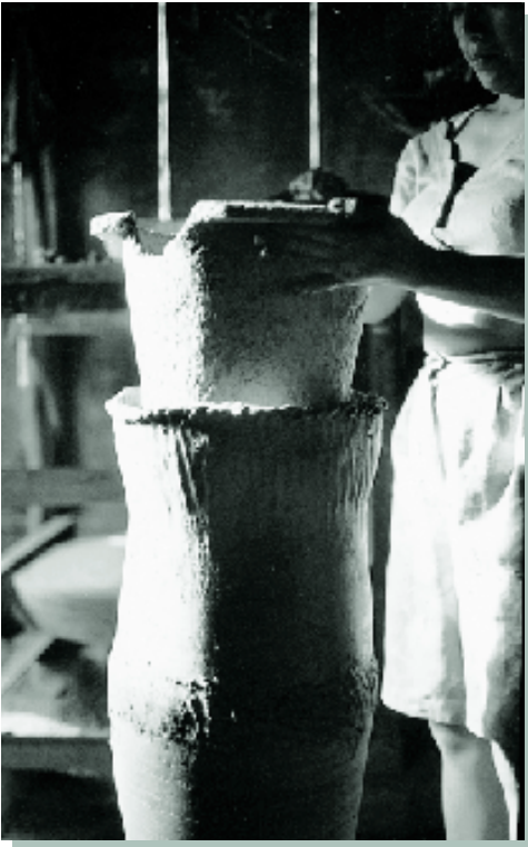
Francis Cano practicing making a water filter receptacle in San Juan de Oriente, Nicaragua.
